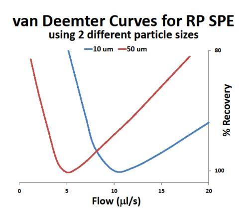
Figure 4. van Deemter curves for reverse phase ( $C_{18}$  endcapped) SPE using two different particle diameters (10 and 50  $\mu$ m). This figure also shows the source of variable recovery with vacuum or pneumatically driven flow, because as flow drifts away from the optimum, there is always a price paid in recovery.
