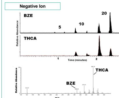
**TOP: Mass chromatograms** for protonated BZE and THCA from duplicate analysis of sample at each concentration
