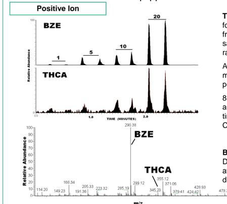
**TOP: Mass chromatograms** for protonated BZE and THCA from duplicate analysis of sample at each concentration ranging from 1 to 20  $\mu$ g/ml
