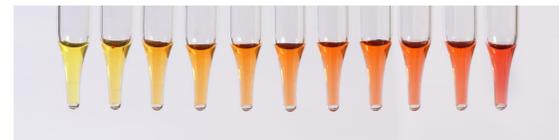
**Step 1. Blend Solvents** – The macro *ITSP SPE MD Blend Solvents* blends two solvents beginning with 100% in position one decreasing to 0% in position 11. Likewise Solvent two starts with 0% in position 1 and ends with 100% in position 11.
