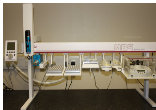
Figure 2 – Gerstel MPS for automated androstenedione and testosterone extraction.
