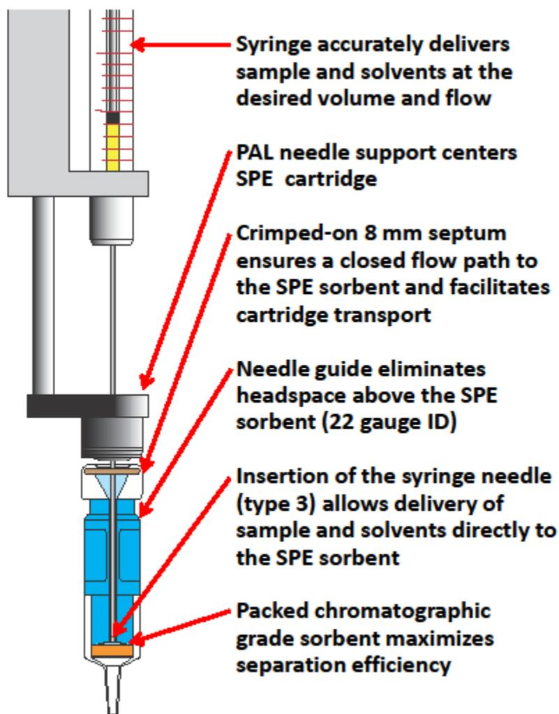
**Figure 1. Internal view of an ITSP SPE cartridge and how it interfaces with the PAL autosampler syringe and needle support. This interface facilitates all SPE cartridge transport and delivery of sample and solvents.**
