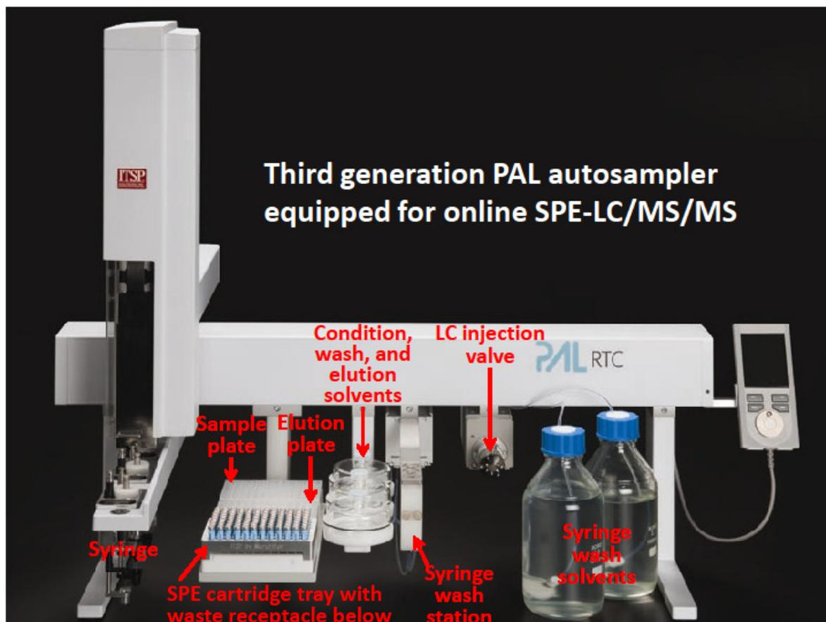
**Figure 2. A PAL RTC autosampler equipped to perform online SPE-LC/MS/MS.**
