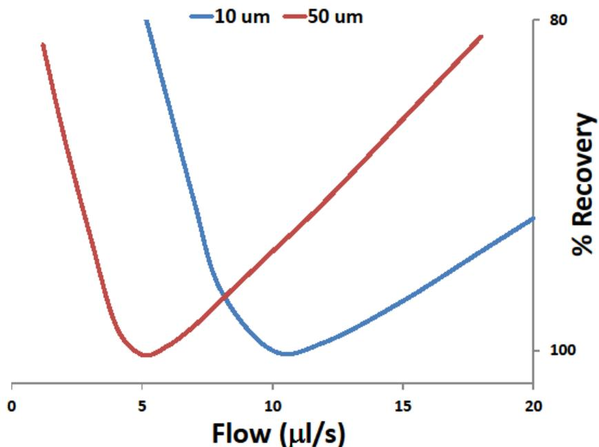
**Figure 4. van Deemter curves for reverse phase ( $C_{18}$  endcapped) SPE using two different particle diameters (10 and 50  $\mu\text{m}$ ). This figure also shows the source of variable recovery with vacuum or pneumatically driven flow, because as flow drifts away from the optimum, there is always a price paid in recovery.**
